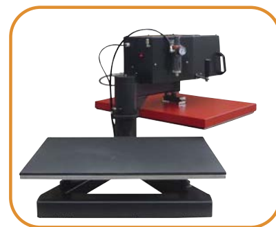
Fig. 2 - freestanding supporting plate
